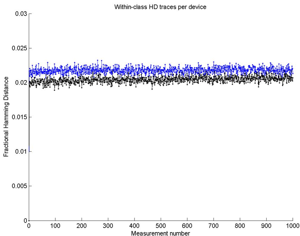
Figure 2.3.18: Within-class Hamming distance of SRAM in Arduino Mega measurements.
