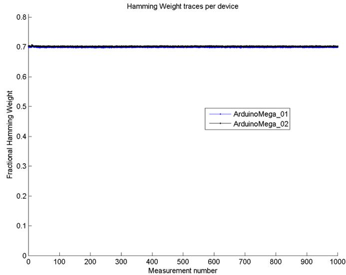
Figure 2.3.20: Hamming weight of SRAM in Arduino Mega measurements.
