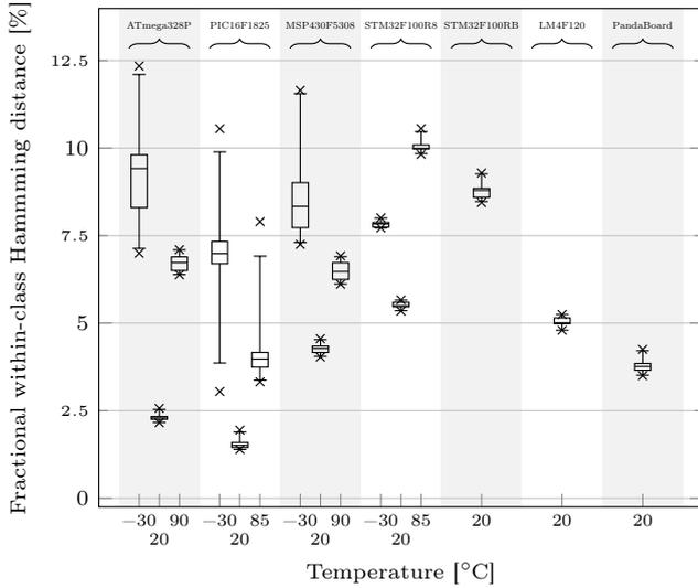
**Fig. 4** Within-class Hamming distance for all measured device types.
