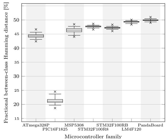
**Fig. 5** Between-class Hamming distances for all measured device types.
