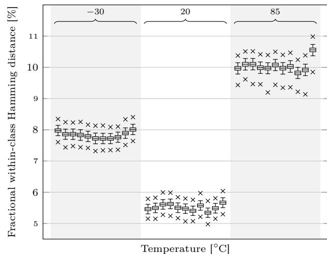
**Fig. 3** Comparison of average Within-class Hamming distances for the individual *STM32F100R8* devices.
