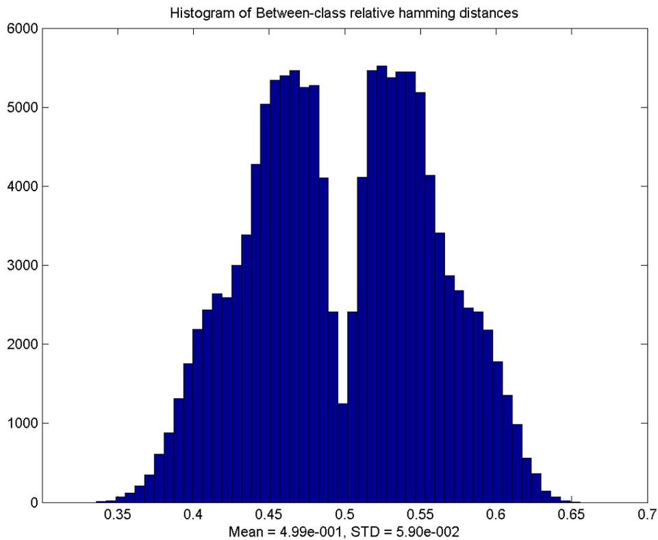
Figure 2.3.7: Between-class Hamming distance distribution of GTX 295 measurements.
