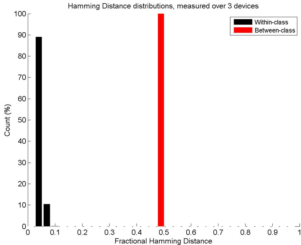
Figure 2.3.15: Between-class versus within-class Hamming distance of SRAM in BeagleBone measurements.
