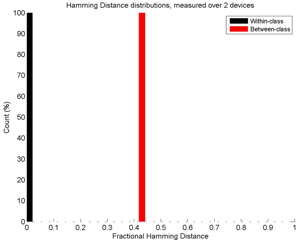
Figure 2.3.19: Between-class versus within-class Hamming distance of SRAM in Arduino Mega measurements.
