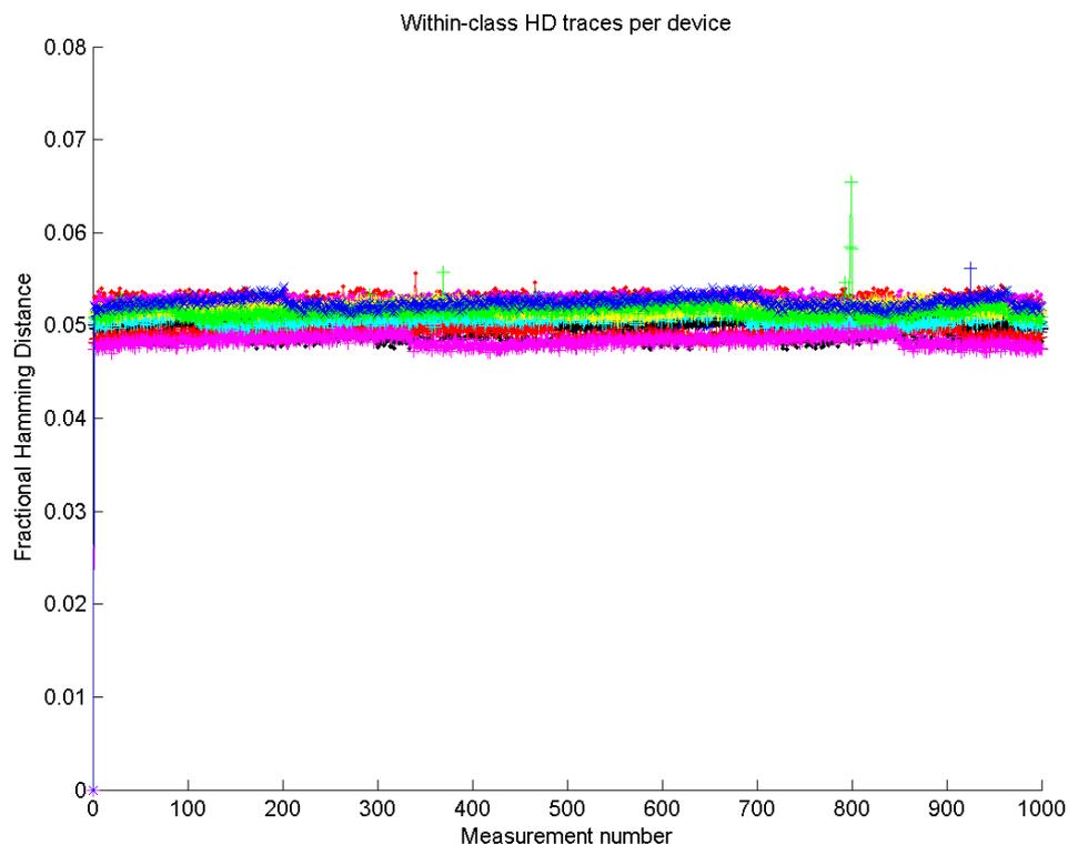
Figure 2.3.10: Within-class Hamming distance of SRAM in LM4F120H5QR measurements.
