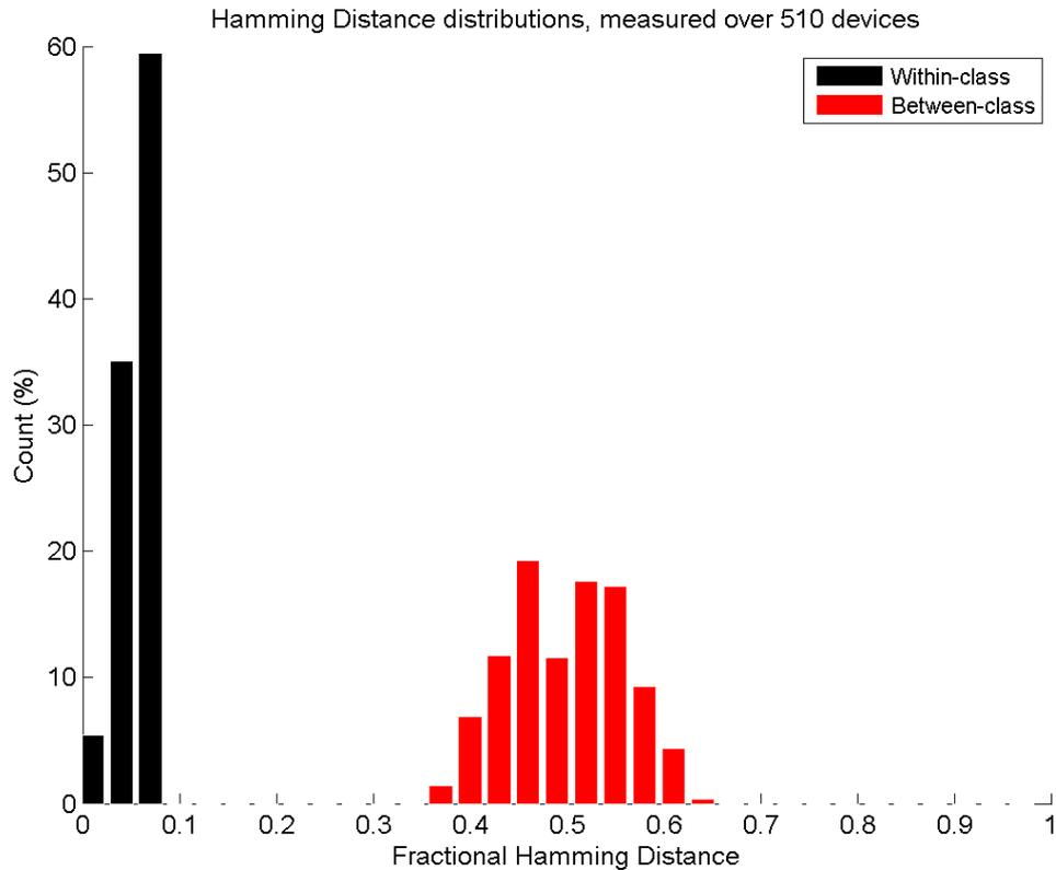
Figure 2.3.6: Between-class versus within-class Hamming distance of SRAM in GTX 295 measurements.
