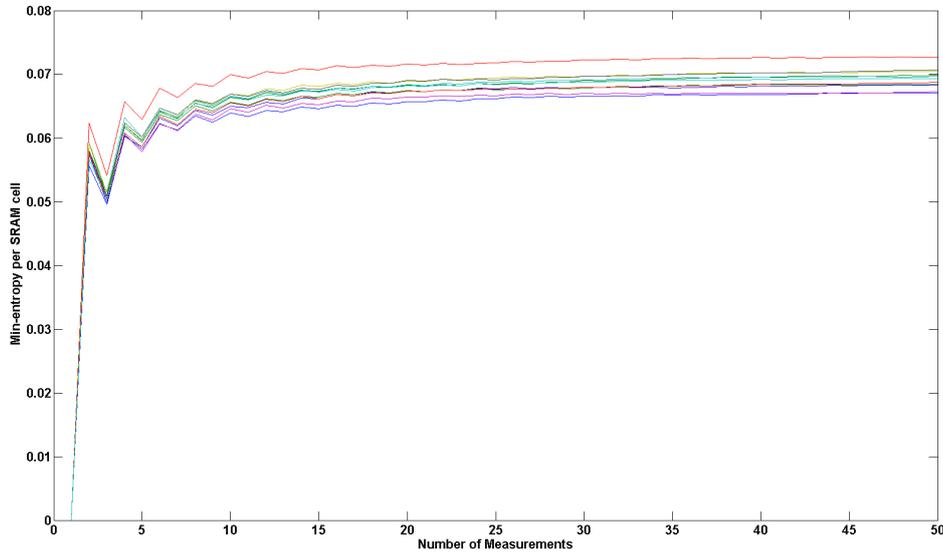
Figure 2.3.22: Min-entropy calculations for STM32F100RB based on 50 measurements.
