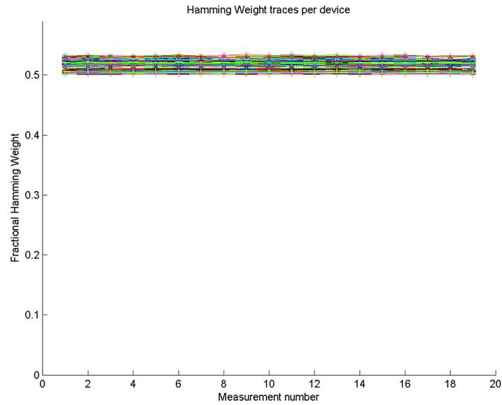
Figure 2.3.8: Hamming weight of SRAM in GTX 295 measurements.
