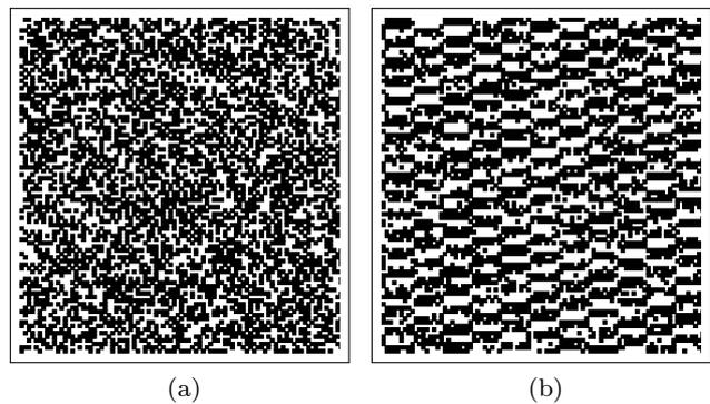
**Fig. 8** Example 1 KiB start-up patterns at 25 °C. Left: *STM32F100R8*, right: *PIC16F1825*. White represents a bit with value 0, black one with value 1.
