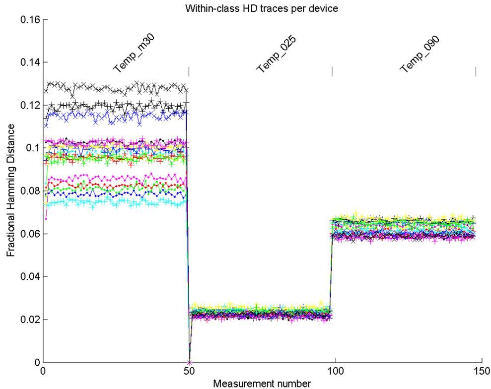
Figure 2.3.4: Within-class Hamming distance of SRAM in ATmega328p measured over different temperatures.
