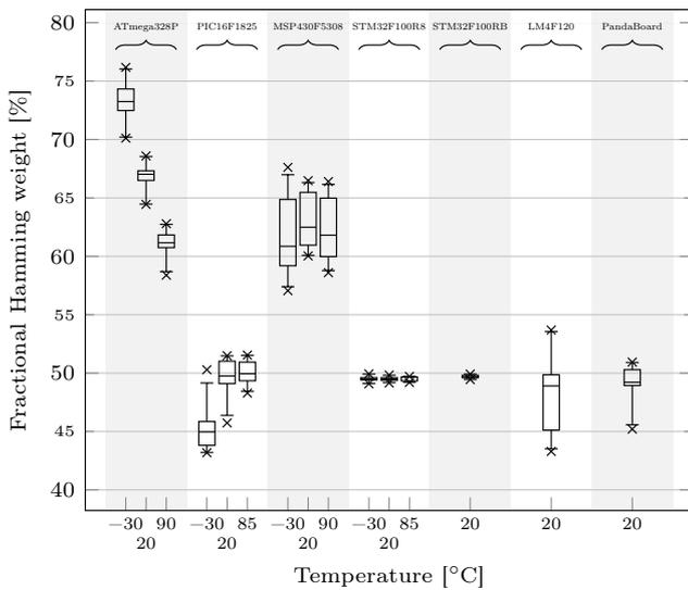
**Fig. 2** Comparison of average Hamming weights among device types.
