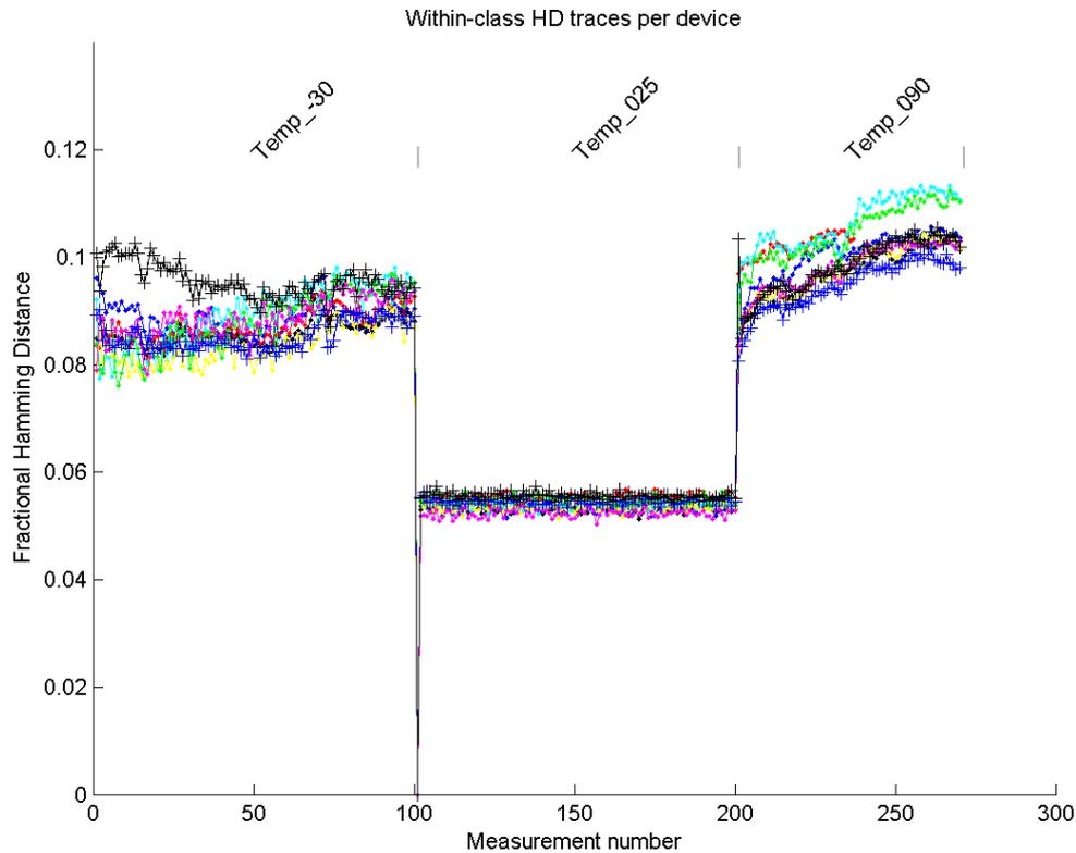
Figure 2.3.3: Within-class Hamming distance of SRAM in STM32F100R8 measured over different temperatures.
