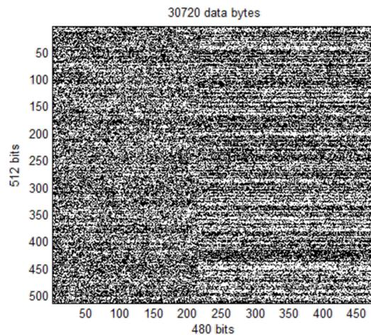
Figure 2.3.17: Example of SRAM PUF response from BeagleBone measurement.
