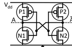
Fig. 1: Cross-coupled CMOS inverter circuit at the core of each SRAM cell. (Two SRAM access MOSFETs not shown.)
