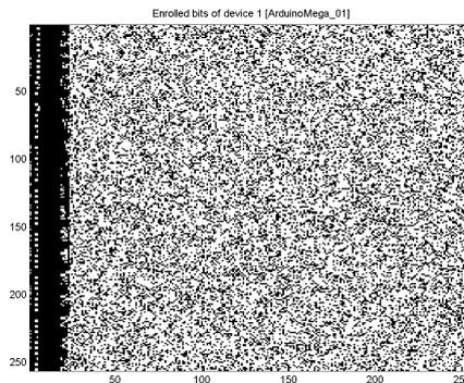
Figure 2.3.21: Example of SRAM PUF response from Arduino Mega measurement.
