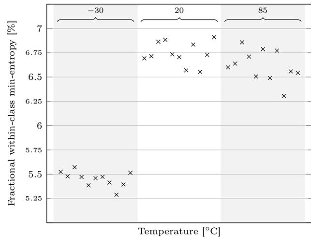
**Fig. 7** Comparison of average fractional min-entropy of the noise extracted from the individual *STM32F100R8* microcontrollers.
