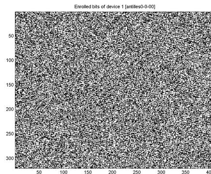
Figure 2.3.9: Example of SRAM PUF response from GTX 295 measurement.
