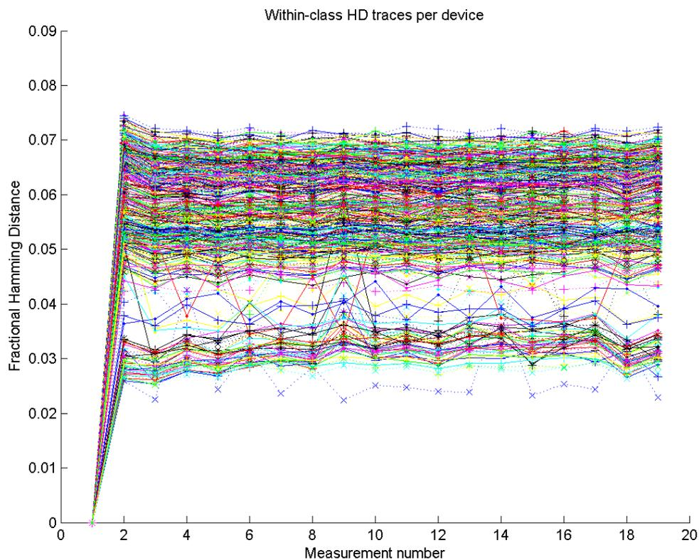
Figure 2.3.5: Within-class Hamming distance of SRAM in GTX 295 measurements.
