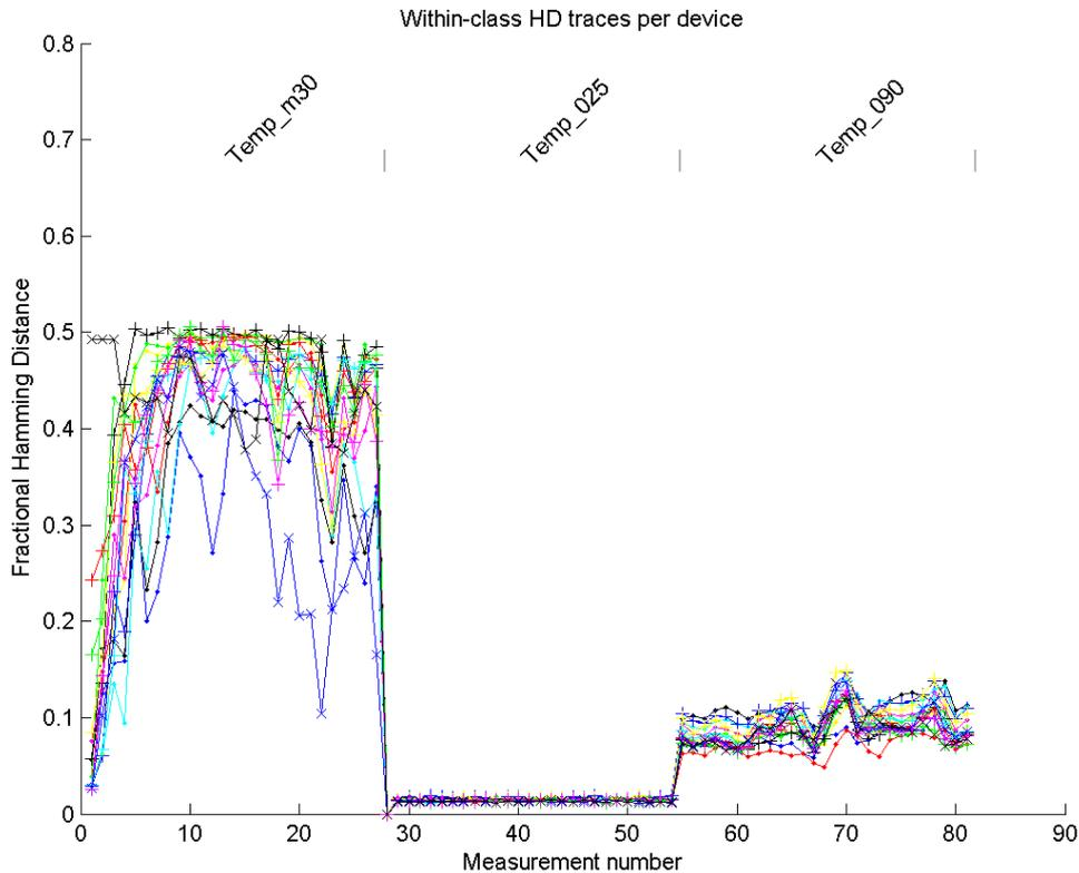
Figure 2.3.1: Within-class Hamming distance of SRAM in PIC16F1825 measured over different temperatures.
