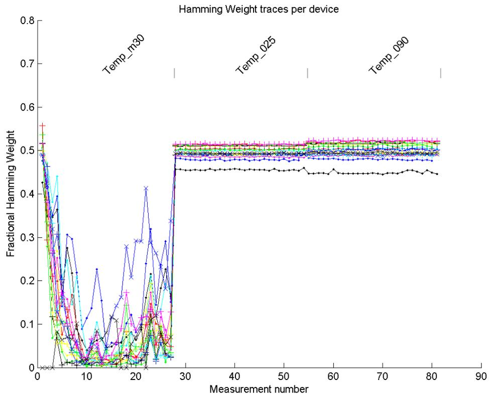
Figure 2.3.2: Hamming weight of SRAM in PIC16F1825 measurements over different temperatures.
