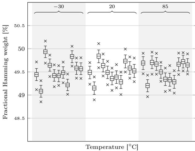
**Fig. 1** Comparison of average Hamming weights for the individual STM32F100R8 devices.
