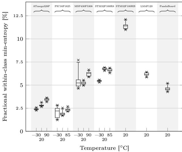
**Fig. 6** Comparison of average fractional min-entropy of the noise exhibited among different device types.
