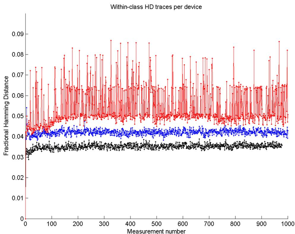
Figure 2.3.14: Within-class Hamming distance of SRAM in BeagleBone measurements.
