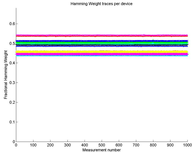
Figure 2.3.12: Hamming weight of SRAM in LM4F120H5QR measurements.
