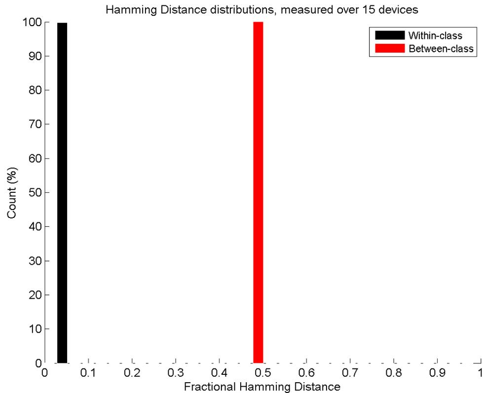
Figure 2.3.11: Between-class versus within-class Hamming distance of SRAM in LM4F120H5QR measurements.
